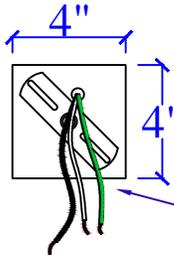
STANDARD 4" ROUND OR SQUARE PANCAKE BOX WITH HANGAR BAR. PANCAKE BOX MUST BE SECURED TO HOLD FIXTURE. USE PROPER ANCHOR BOLTS/LAG BOLTS
