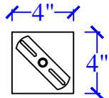
STANDARD 4" ROUND OR SQUARE PANCAKE BOX WITH HANGAR BAR. PANCAKE BOX MUST BE SECURED TO HOLD FIXTURE. USE PROPER ANCHOR BOLTS/LAG BOLTS
