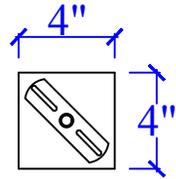
STANDARD 4" ROUND OR SQUARE PANCAKE BOX WITH HANGAR BAR. PANCAKE BOX MUST BE SECURED TO HOLD FIXTURE. USE PROPER ANCHOR BOLTS/LAG BOLTS
