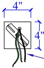
STANDARD 4" ROUND OR SQUARE PANCAKE BOX WITH HANGAR BAR. PANCAKE BOX MUST BE SECURED TO HOLD FIXTURE. USE PROPER ANCHOR BOLTS/LAG BOLTS
